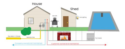
If corrosion or other unsafe conditions are found, the pipes should be repaired immediately. Contact your local plumbing/heating contractor to have your gas lines checked or visit the safety page of our website for more information about customer-owned piping.
